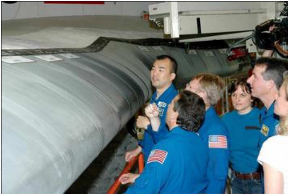
In the Orbiter Processing Facility, members of the STS-114 crew take a close look at the Reinforced Carbon-Carbon on the wing's leading edge on Discovery.
