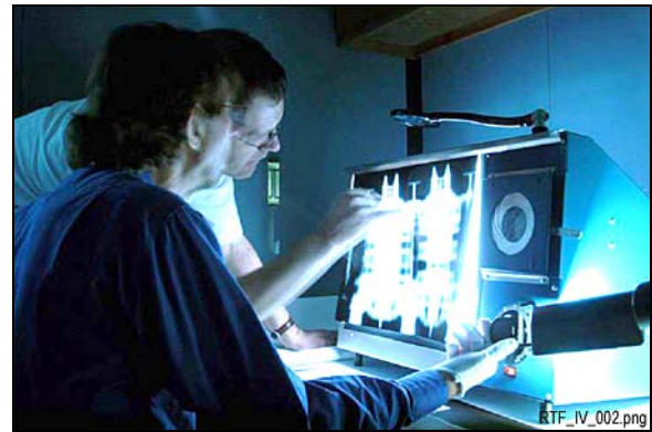
Actuator inspection using X-ray analysis
