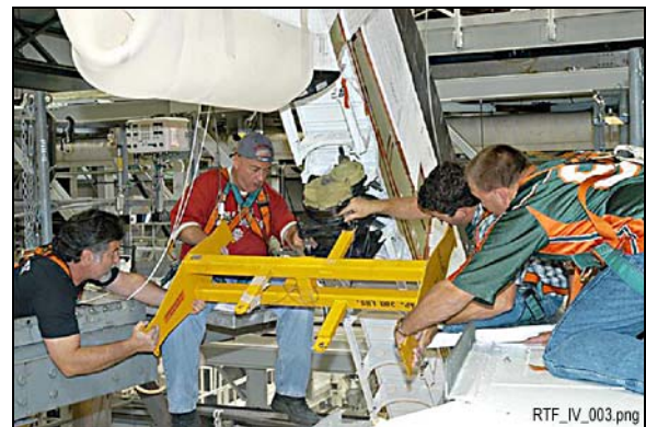
Actuator installation on Discovery
